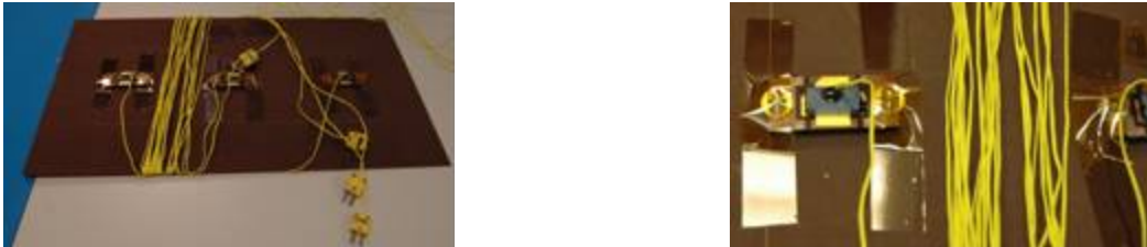
Figure 7 – The three devices with captors on the top of the packages to create the temperature profile
